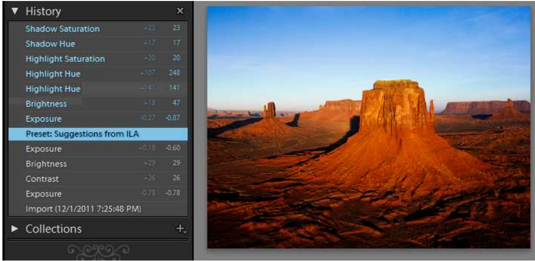
Figure 5: The planned interface. The History window shows the series of adjustments in chronological order, from bottom to top. After the user chooses to get suggestions from the ILA (shown with a blue background in the History window), a series of new adjustments will be displayed (typeset in blue). The user can then click through each adjustment to see what was changed, or accept the final result and ignore the intermediate steps.
