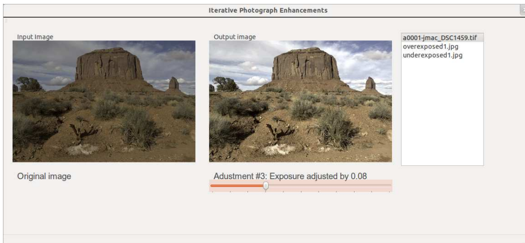
Figure 4: The current interface. As the user moves the slider to the right, successive iterations are displayed. The text above the slider describes the adjustment that brought the user from the previous state to the one shown.
